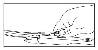
Install the new blade onto the arm connector and make sure the grooved areas are fully set in the locked position.
